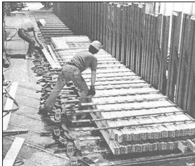
Figure 1 – Manual clamping of straight beams (MARRA)
